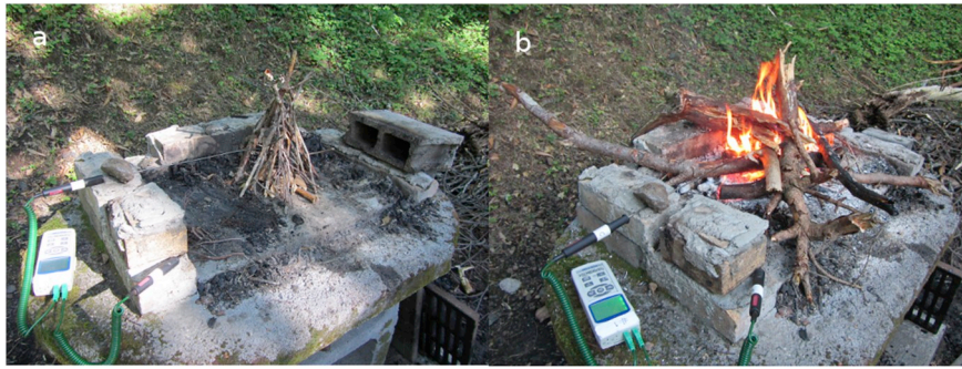
Fig. 3. Fire pit set up. a) before lighting the fire. b) during the burning.
