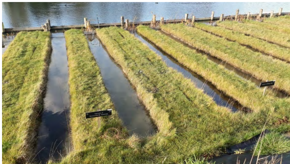
Figure 6.2. Photographic overview of the experimental site ‘the Living Lab’. Top to bottom: adjoining reservoir, wave barrier, macrophytes, netting, experimental ditches.
