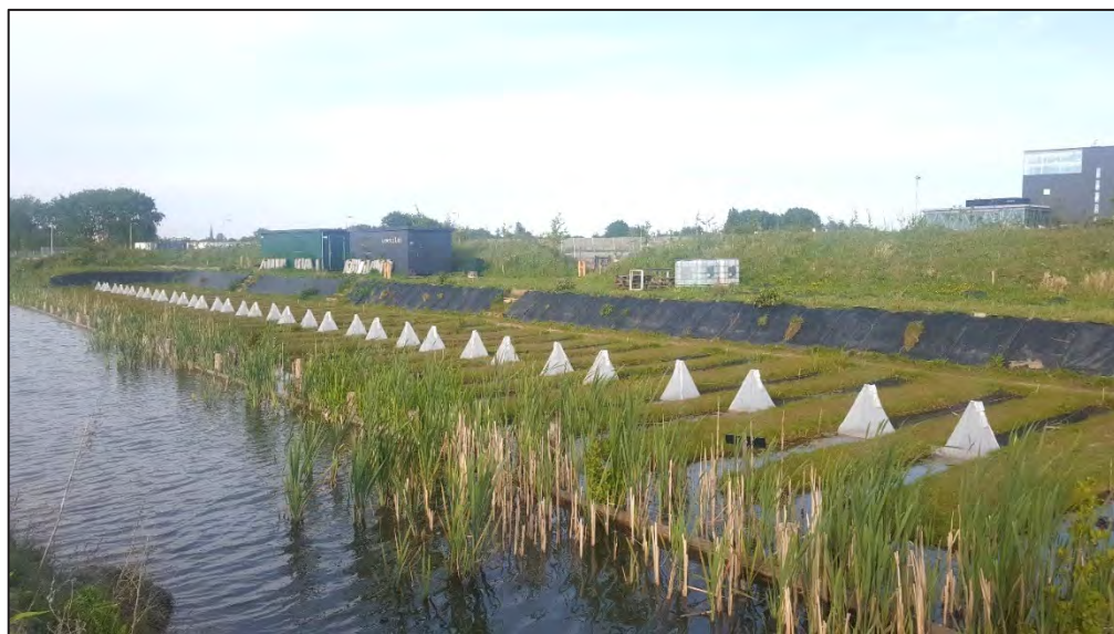
Figure 3.S1. Photographic overview of the experimental site. From left to right: adjoining lake, wooden wave barrier, helophytes, experimental ditches. The white pyramids are the emergence traps used in the present study.
