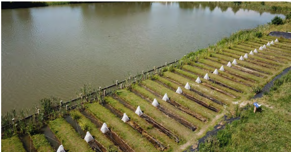
Figure 7.1. Top-view of the experimental ditch system. Top-left to bottom-right: adjoining lake, wave barrier, helophyte layer, netting, hydrological barrier, experimental ditch.
