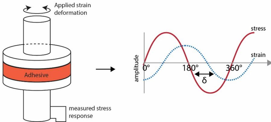
**Fig. 5.** Schematic showing sample and output data from the rheometer. Left: the adhesive sample between the upper and lower plates of the rheometer and the force oscillating about the y-axis (not to scale). Right: the resulting oscillating stress/strain curve. For ideally viscous liquids  $\delta = 90^\circ$  and ideally elastic solids  $\delta = 0^\circ$ .
