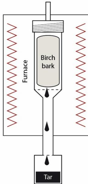
**Fig. 2.** Schematic of tube furnace heating apparatus used to distill birch bark tar. The work-tube and screen to hold the bark are made of stainless steel with a small outlet at the top to relieve pressure in the event that the lower pipe should become blocked. Not to scale.
