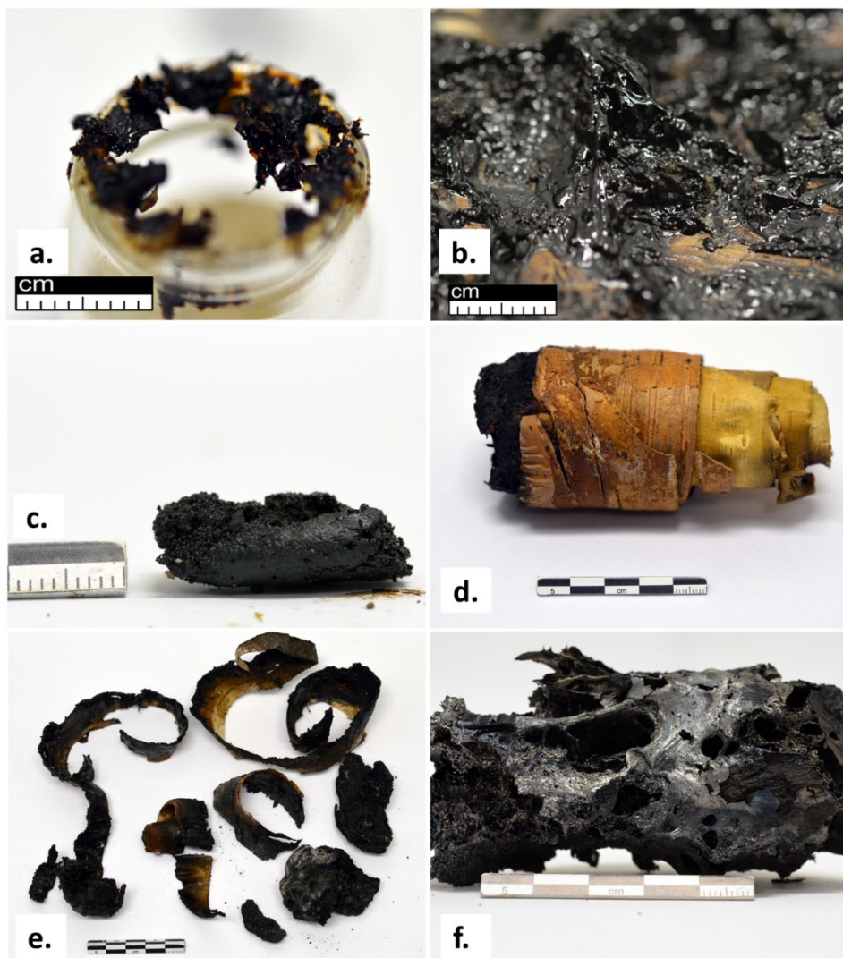
Supplementary Figure S13. Photographs of the remains of various methods and products. a) Some tar from the ash mound method that is highly contaminated with traces of un-charred birch bark; b) tar from the RS7 vessel containing very few contaminants; c) lump of tar from RS8 (using a shell vessel) heavily contaminated in soil. It holds its form, but has very little tack due to the over-saturation of particles; d) remains of bark roll from PR 3 and PR 4. Only slight charring at the end that was ignited and the rest is unchanged; e) remains of bark from successful PR experiment contains much more charred bark; f) bark remains from raised structure RS7. The bark is highly charred and does not resemble birch bark macroscopically.
