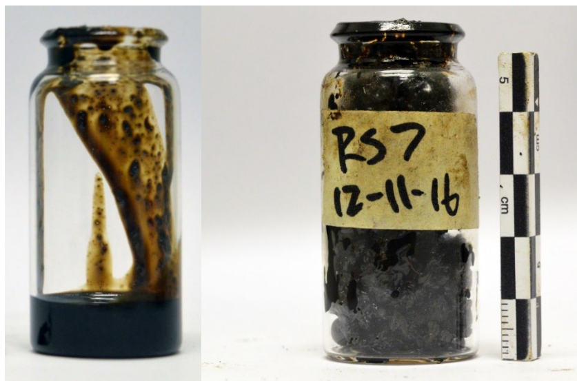
Supplementary Figure S14. Tar from RS 4 (left) and RS 7 (right). RS 4 used a metal container to collect the tar. Temperatures were higher in the metal container (refer above to Fig. S13), but the tar collected remained more liquid than that from RS 7. Suggesting some of the more liquid portion of tar is lost to the earth pit walls, or to the organic vessel.
