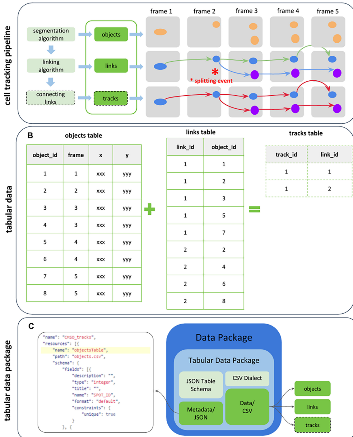
Figure 4: Schematic view of the biotracks format developed by the CMSO. In A , a segmentation algorithm identifies objects in the raw images, annotating them with the frame information, coordinates, and any other features that the algorithm extracts. These are described in the objects table in B . A linking algorithm then connects the objects across frames in a parent-child relationship. Among the possible events, the linking algorithm can then identify a split, where a parent has >1 child. This information is reported in the links table in B . The tracks table in B can finally be inferred from the objects and links tables. The tabular data package format is represented in C . Here, objects, links, and tracks data tables are saved as comma-separated values (CSV) files. The accompanying file in the JSON format contains both the general metadata of the data package and the metadata of the CSV files.
