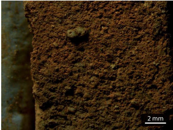
Figure 202: Sample RDO2.B4, featuring prominent grains characteristic of wet clay finishing.
