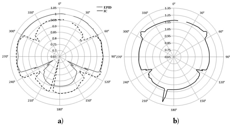
**Figure 3.4.** a) The output factor at the isocenter (solid-grey) and at EPID level (dashed-black) as function of the gantry angle and normalized to the measurement at 90 degrees. b) The normalized ratio of IC/EPID.
