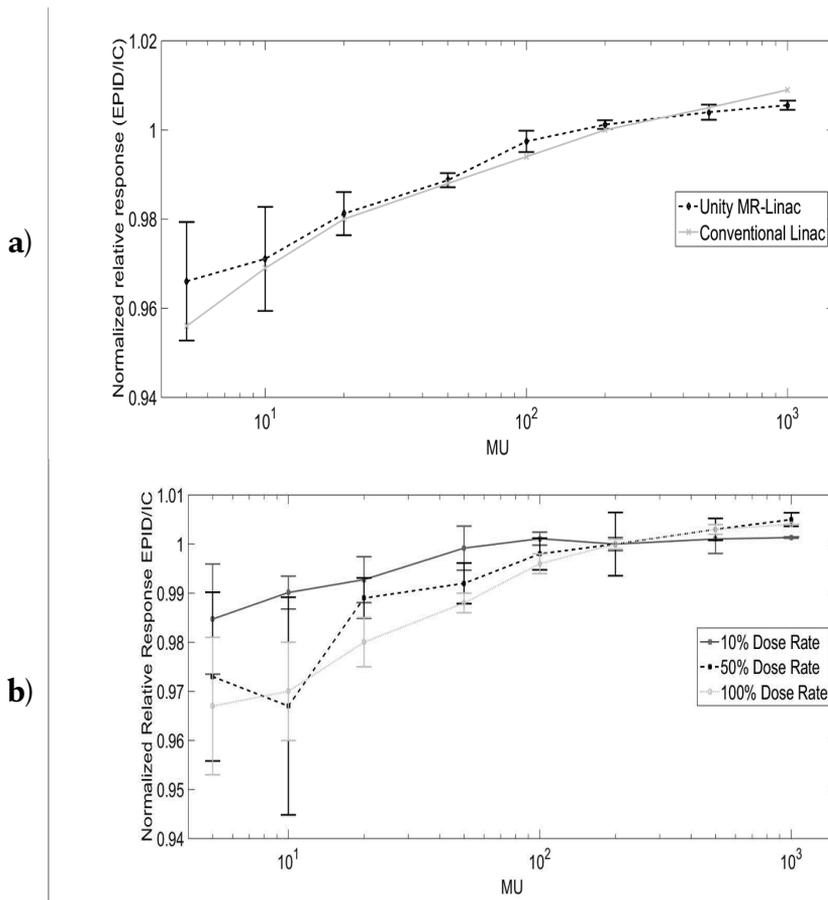
**Figure 3.6. a)** The relative EPID response (EPID/IC) as a function of dose for a varying number of MUs is plotted for the MR-linac (dashed-black) and in a conventional linac (solid-grey), normalized to the 200 MU point. Variations of the EPID signal divided
