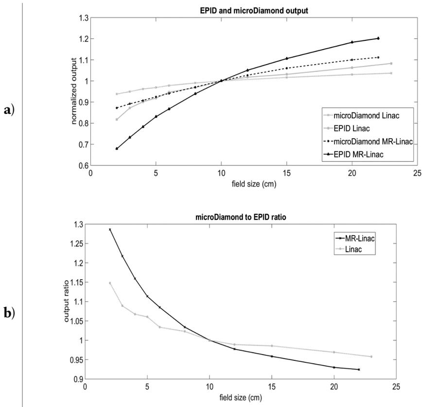
**Figure 3.3.** **a)** Field size dependence of microDiamond detector measurements at the EPID level (dashed line) and averaged EPID signal over the central 10x10 pixels (solid line) for the MR-linac system (black) and a conventional linac (grey); **b)** the output ratio of the microDiamond detector to the EPID signal is plotted for both the conventional linac (dashed grey) and the MR linac (solid black).
