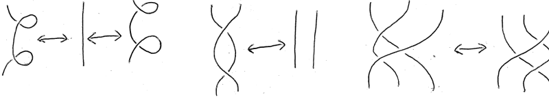
Figure 3.2.: The Reidemeister moves for a framed knot. From left to right the Reidemeister I, II and III move.
