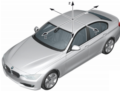
Figure 2.2: The vehicle coordinate system. (Original photo from BMW Group Technical Qualification Media)
