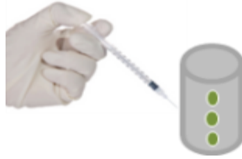
Figure 3.1. The injection protocol with green spots indicating the injection position of fluorescence spheres. The cylinder corresponds to the shape of the agarose block as mounted in the OPT.
