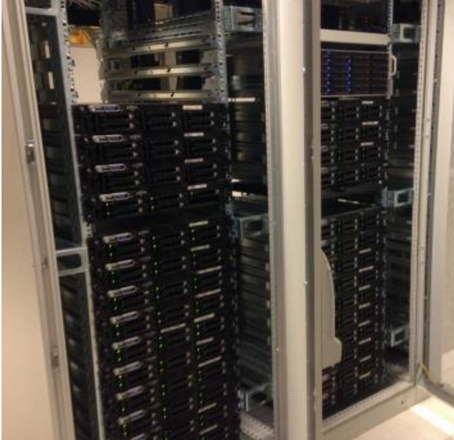
Figure 2.2. The LLSC cluster with three user nodes, 20 computing nodes (108 processors) and a file server.
