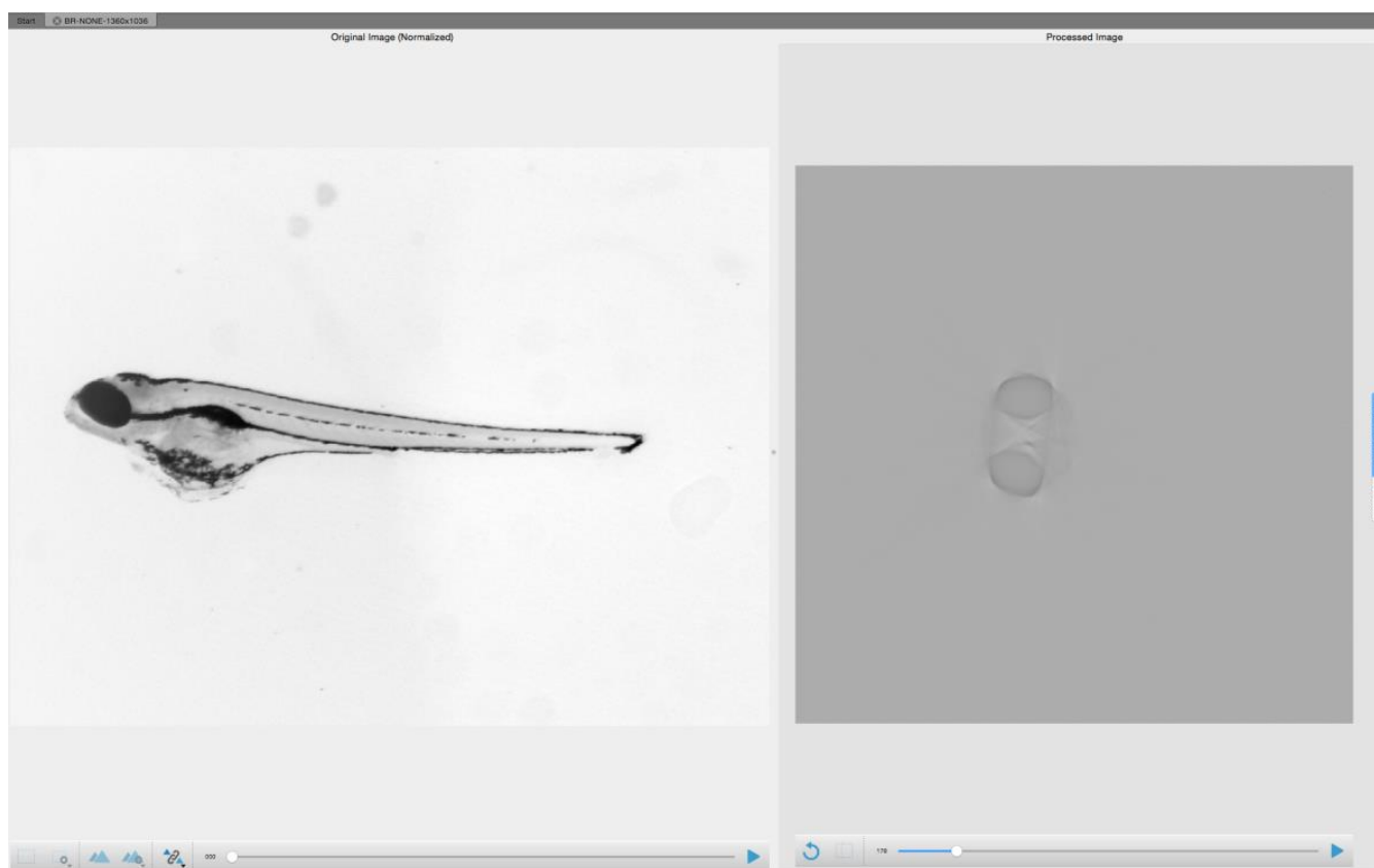
Figure 2.1. The user interface of the post-processing software; it includes cropping, background subtraction, CoR correction and 3D reconstruction. Once the tomogram is opened, cropping and background subtraction can be done with buttons on the left. With a Start Reconstruction button, the data are automatically uploaded to a dedicated cluster computer. The CoR correction and reconstruction are distributed on the cluster. The reconstructed results and maximum intensity projections are sent to the local computer after completion (right panel).
