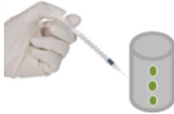
Figure 3.1. The injection protocol with green spots indicating the injection position of fluorescence spheres. The cylinder corresponds to the shape of the agarose block as mounted in the OPT.
