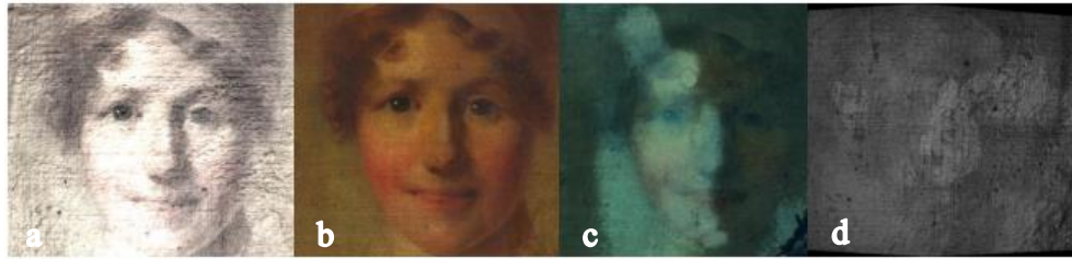
Figure 6-I. (a) RTI, (b) VIS, (c) UVF, (d) CGT gloss map of the face of the sitter. CGT gloss map indicates glossier surface in areas that appear lighter in the image.
