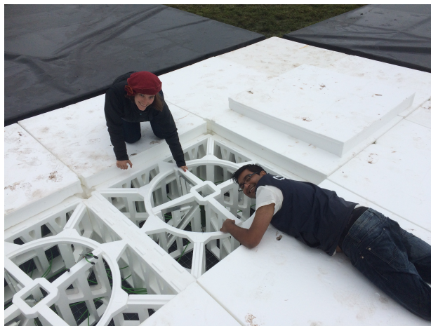
Figuur 6 Field work on LOFAR antenna CS013 on October 22, 2015, a high band antenna. Each square contains a low frequency dual-polarization dipole.
