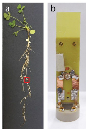
Figure 4.1 Photograph of M. truncatula root system and custom-designed home-built microcoil. (A) Photograph of a representative M. truncatula plant (five weeks old, three weeks post inoculation). Typical root nodule indicated with a red square. Some white perlite beads are still visible along the root system. (B) Photograph of a home-built solenoid coil insert mounted on a Bruker insert holder. The solenoid inner diameter is 1.5 mm; further details are described in the materials and methods.
