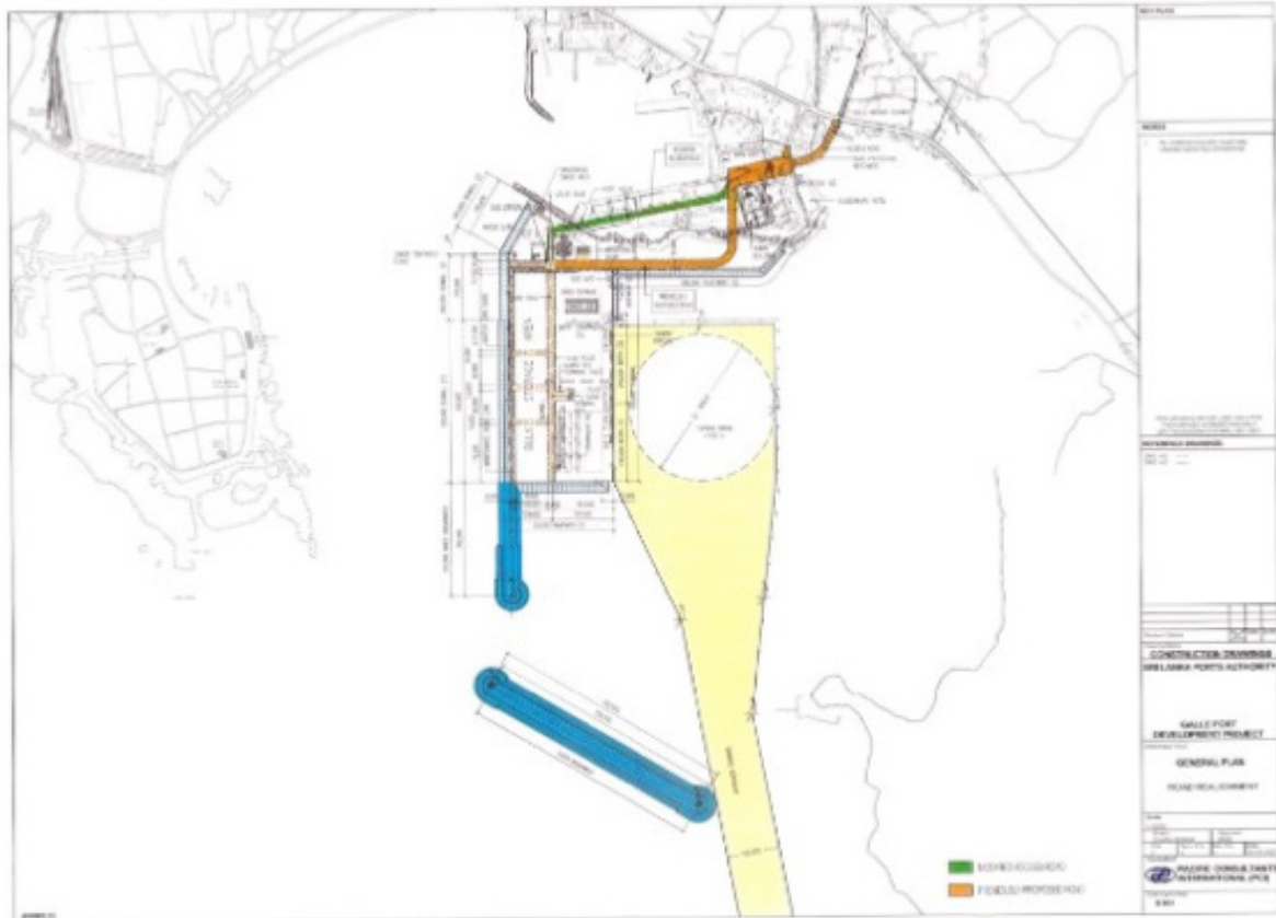
Fig. 281 The revised plan with the proposed new road (in orange), which replaced the initial one (in green) to avoid the wreckage of the East Indiaman Hercules (SLPA 2013).
