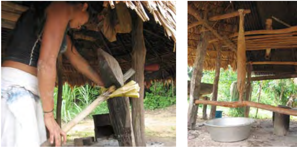
Fig. 3.20: Processing Posts (PPs) in action. (L) A sugarcane press (PP) in ST-26. (R) A manioc squeezer and its position in the leverage construction (PP on the left side) in ST-10.
