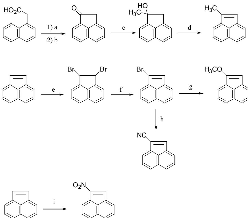
**Scheme 3:** Syntheses of 1-substituted acenaphthylenes, a:  $\text{ClCOCOCl}$ , b:  $\text{AlCl}_3$ , c:  $\text{MeLi}$ , d:  $p\text{-TSA}$ , e:  $\text{Br}_2$ , f:  $\text{KOH}$ , g:  $\text{CuI}$ ,  $\text{NaOMe}$ , h:  $\text{CuI}$ ,  $\text{KCN}$  i:  $\text{AgNO}_3$ ,  $\text{NaNO}_2$ ,  $\text{I}_2$ .
