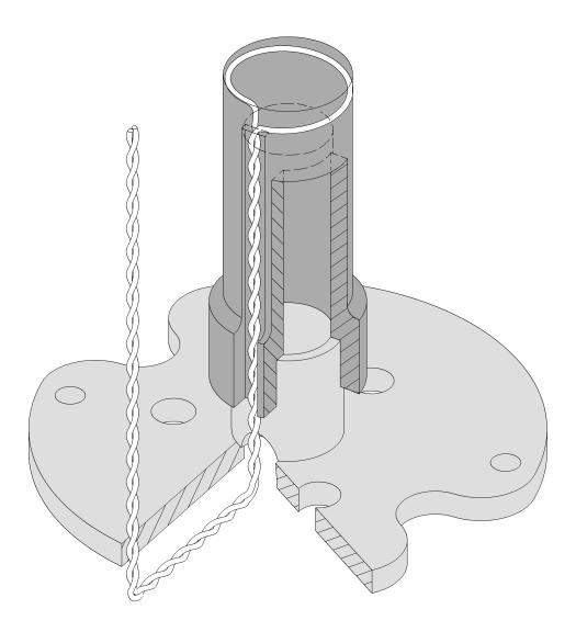
**Figure B.1:** Technical drawing of the revised modulation coil mount. Light gray: Bronze. The bottom plate is attached to the end of the probe head. Dark gray: Stycast. The modulation coil is encased in Stycast. For clarity only one turn is depicted.
