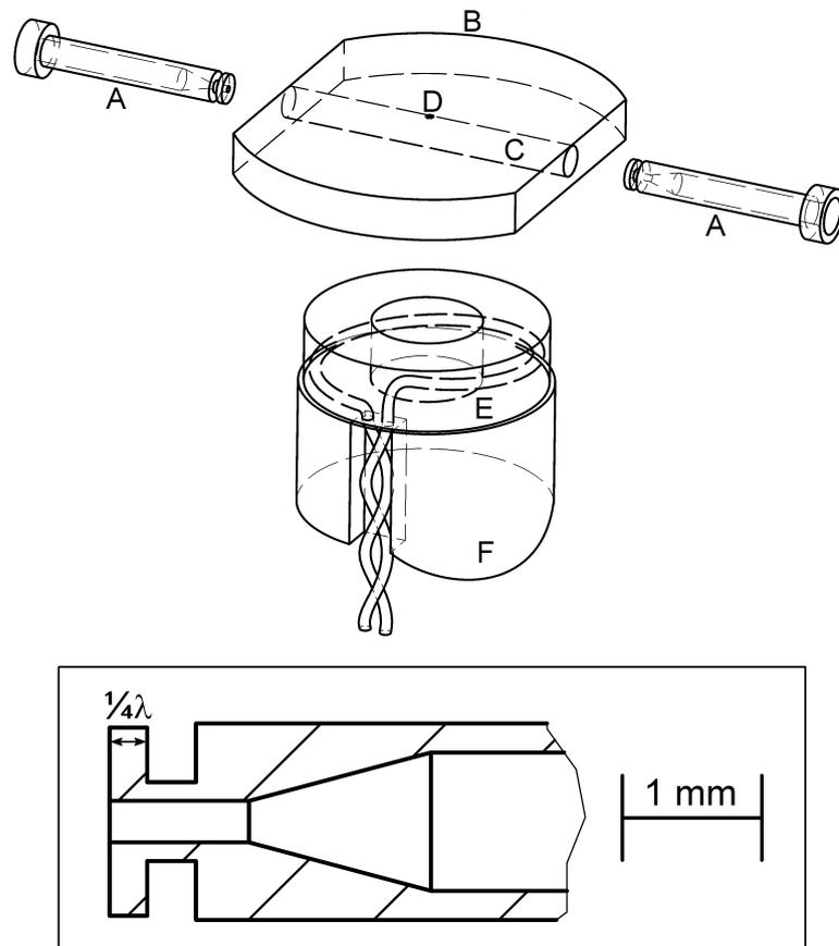
**Figure 2.1:** Schematic drawing of the 275 GHz cw cavity and the modulation coil. A: plungers, B: cavity block, C: cavity, D: coupling hole, E: modulation coil encased in Stycast (for clarity only one turn is depicted) F: modulation coil mount. The inset shows the choke joint at the end of the plungers in detail.
