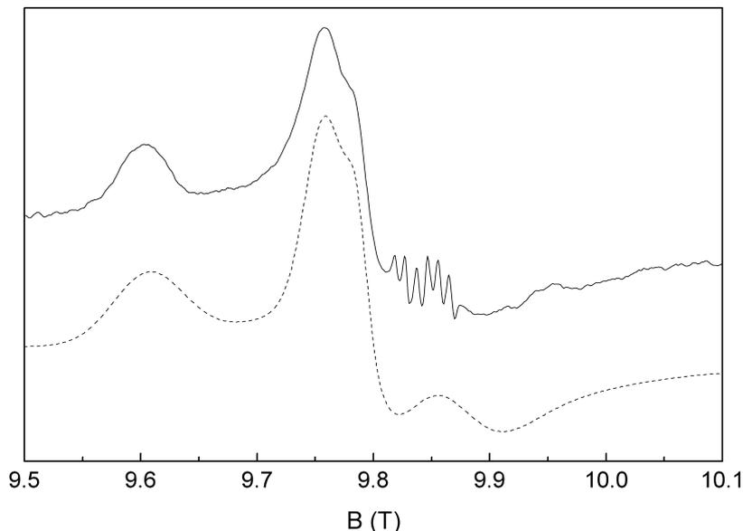
**Figure 2.4:** Detail of the 275 GHz cw EPR spectrum of a 1 mM frozen solution of the model complex Fe(III)-EDTA at 15 K in Figure 2.3. The solid line is the experimentally observed spectrum and the dashed line is the spectrum calculated by EasySpin with the parameters given in Table 2.1.
