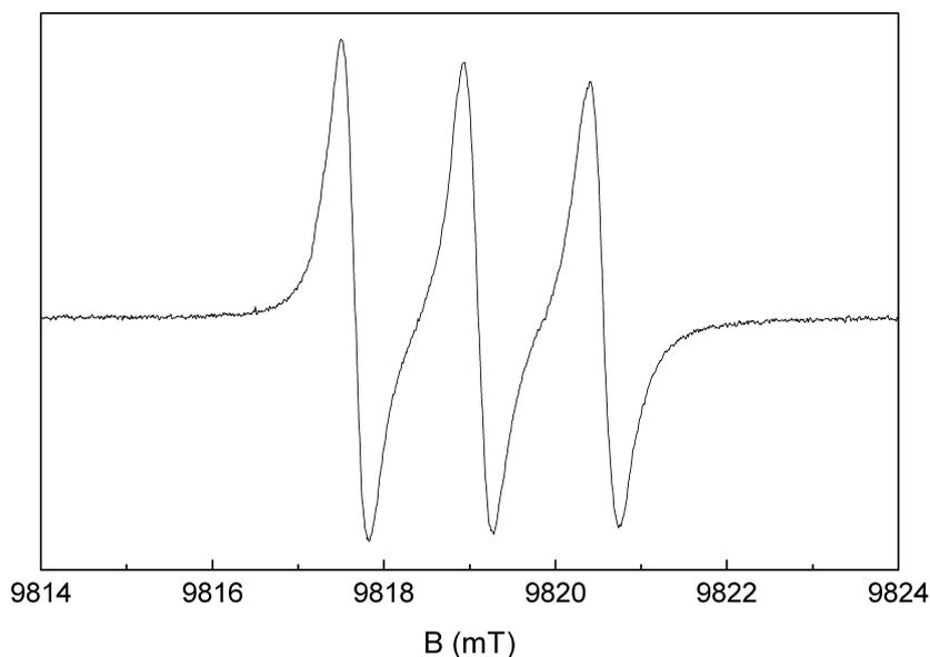
**Figure 2.2:** The room temperature cw EPR spectrum at 275 GHz of a  $10^{-4}$  M solution of the spin label TEMPO in toluene. Experimental conditions: modulation amplitude: 0.05 mT, time constant: 100 ms, microwave power:  $50 \mu\text{W}$ .
