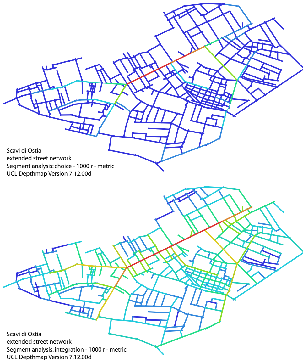
Fig. 7.10 – The metrical radius of 1000 m measured for choice indicates the routes selected by most journeys to reach any destination within the range of the radius of 1000 m; measured for integration, the graph indicates in red the streets which were most accessible to all others and hence most likely selected as destination streets; a high consistency between choice and integration is observable along the eastern decumanus
