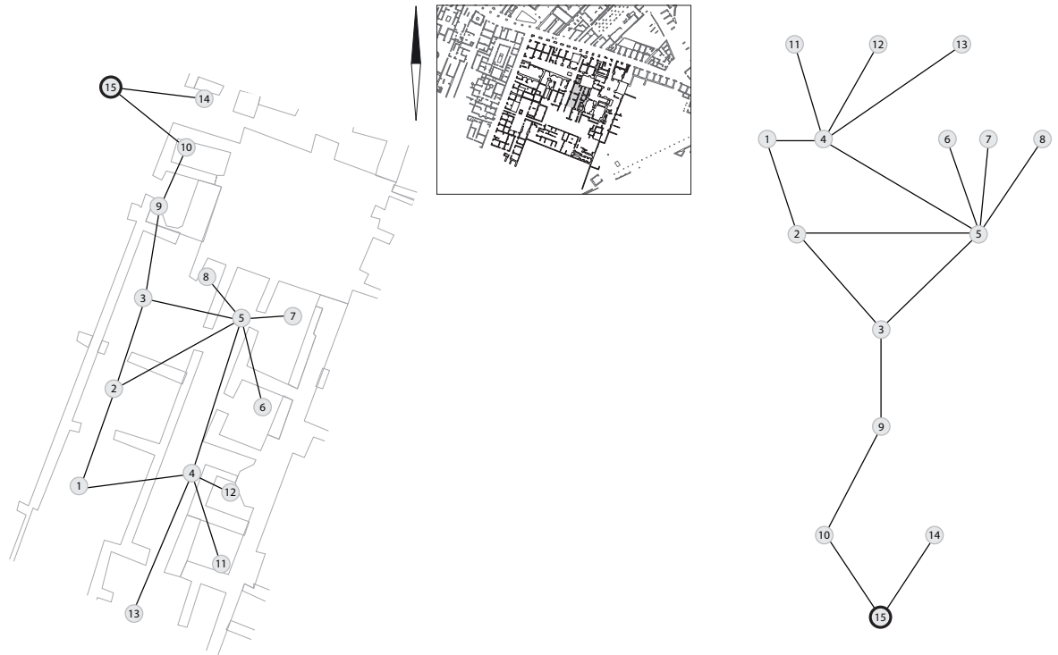
Fig. 6.8 – Caseggiato IV ii 5, J-graph, (root 15 = courtyard) and topological graph (15 = courtyard, 13 = neighbour Building IV ii 12)
