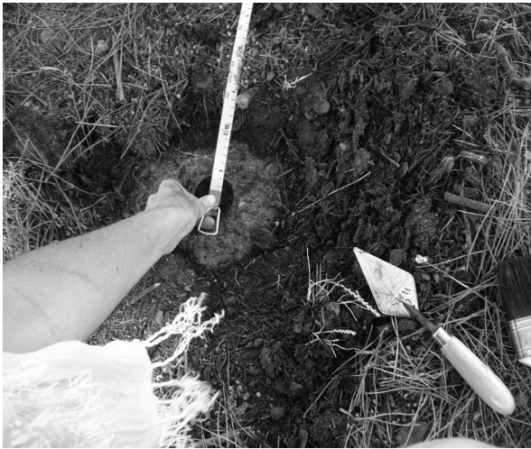
Fig. 4.3 – Local reference points hidden under soil cover, intended for protection from vandalism and amateur excavators
