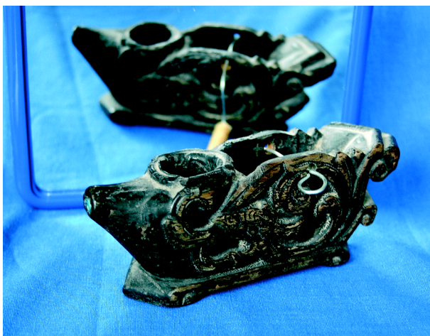
Photograph 1-11 A modou , 墨斗, carpenters' tool used for drawing long lines. A thin rope on the reel would run through the container inside and is coated with ink or chalk.
