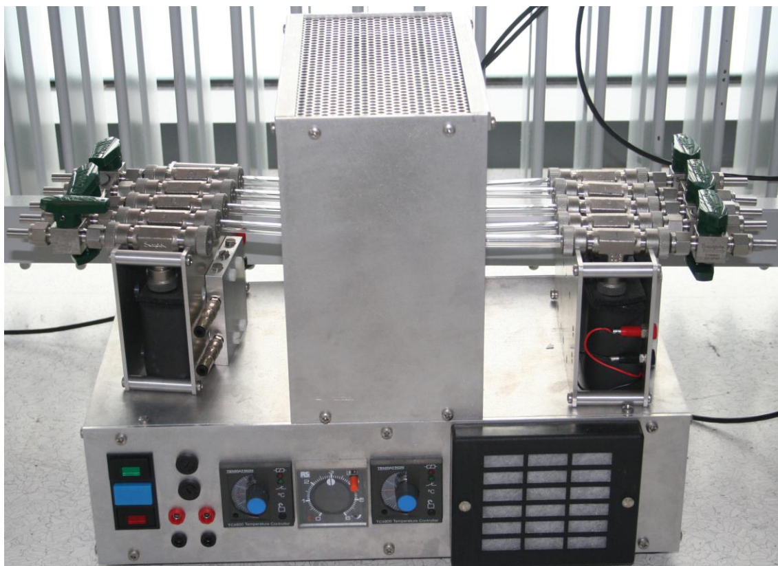
Figure 4.10 Reduction of CO 2 to graphite using iron as catalyst in an oven (top section); water vapour is removed by immersing the vertical finger of the rig into a cooling bath (left and right section).
