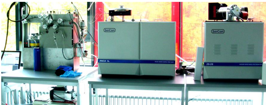
Figure 4.4 Elements of the graphitization: combustion in the EA (middle), \delta^{13}\text{C} and \delta^{15}\text{N} determination in the mass spectrometer (right) and the graphitizer (left).
