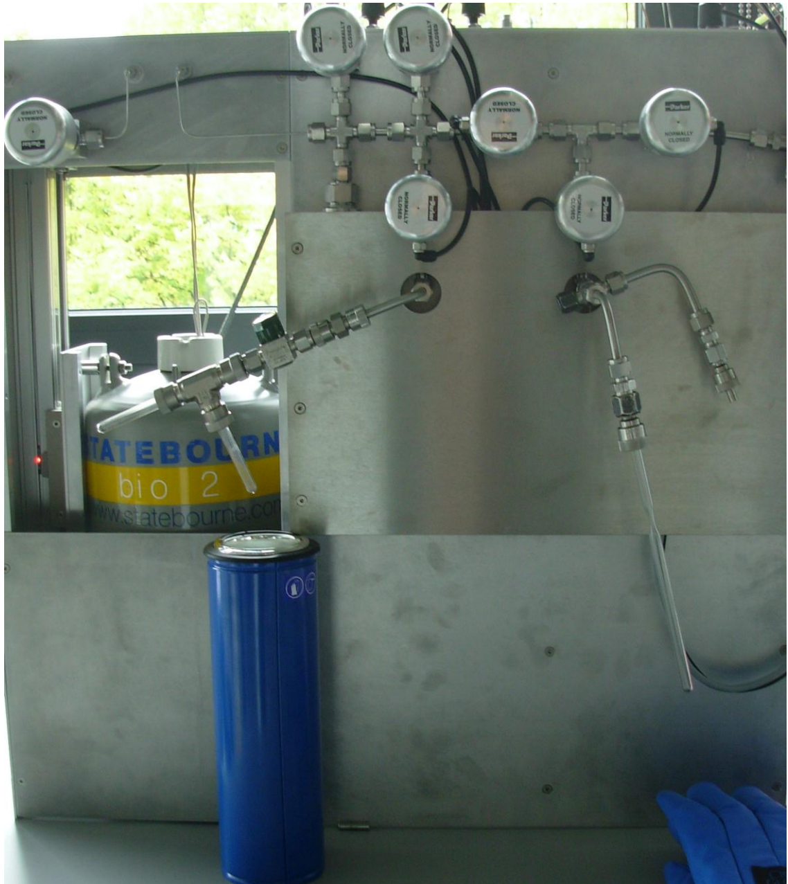
Figure 4.9 Graphitization system manufacture by the Oxford laboratory
