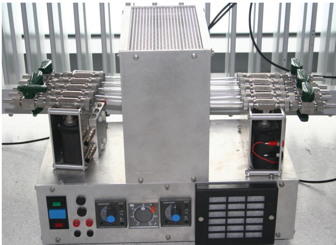
Figure 4.10 Reduction of \text{CO}_2 to graphite using iron as catalyst in an oven (top section); water vapour is removed by immersing the vertical finger of the rig into a cooling bath (left and right section).
