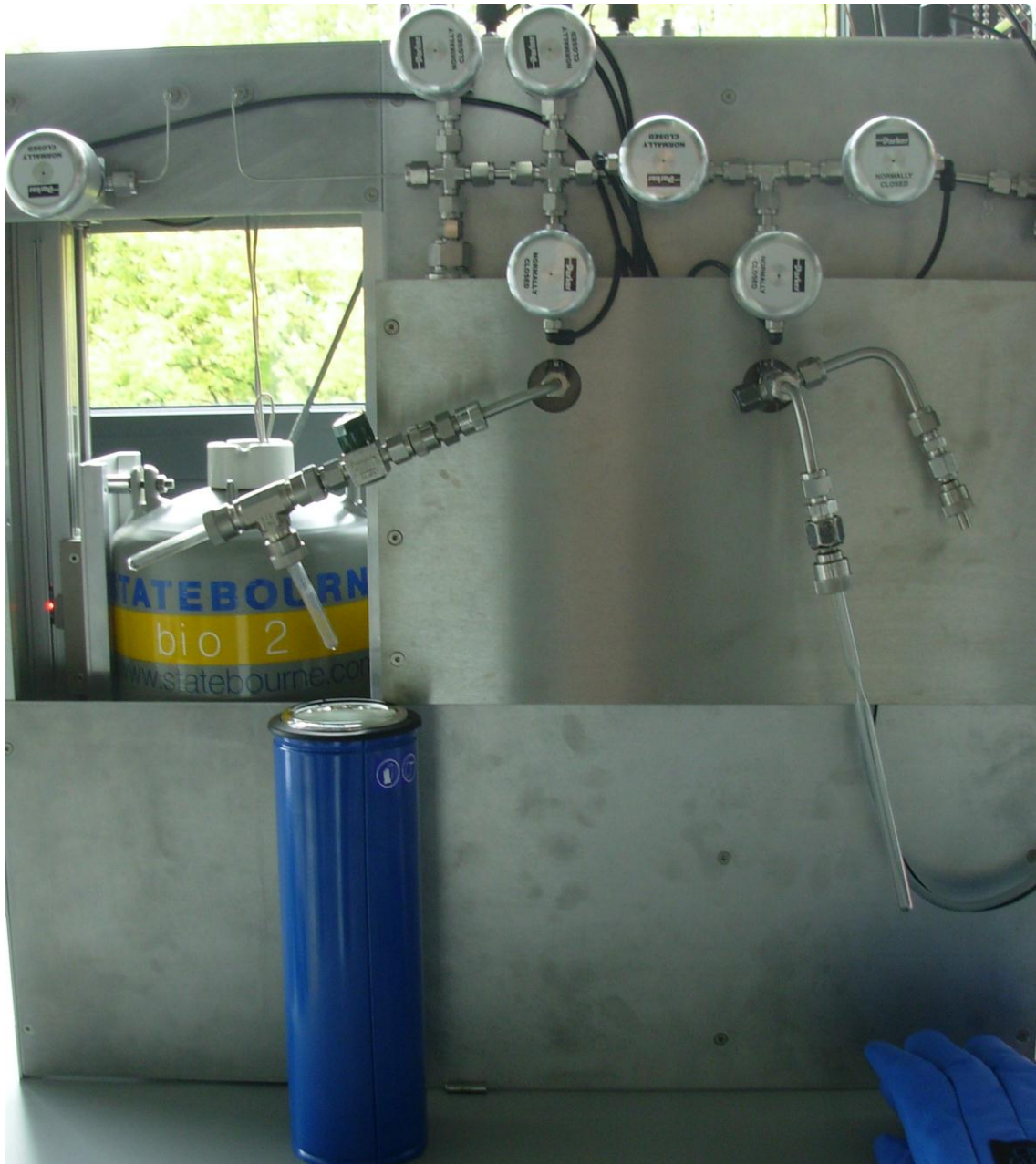
Figure 4.9 Graphitization system manufacture by the Oxford laboratory
