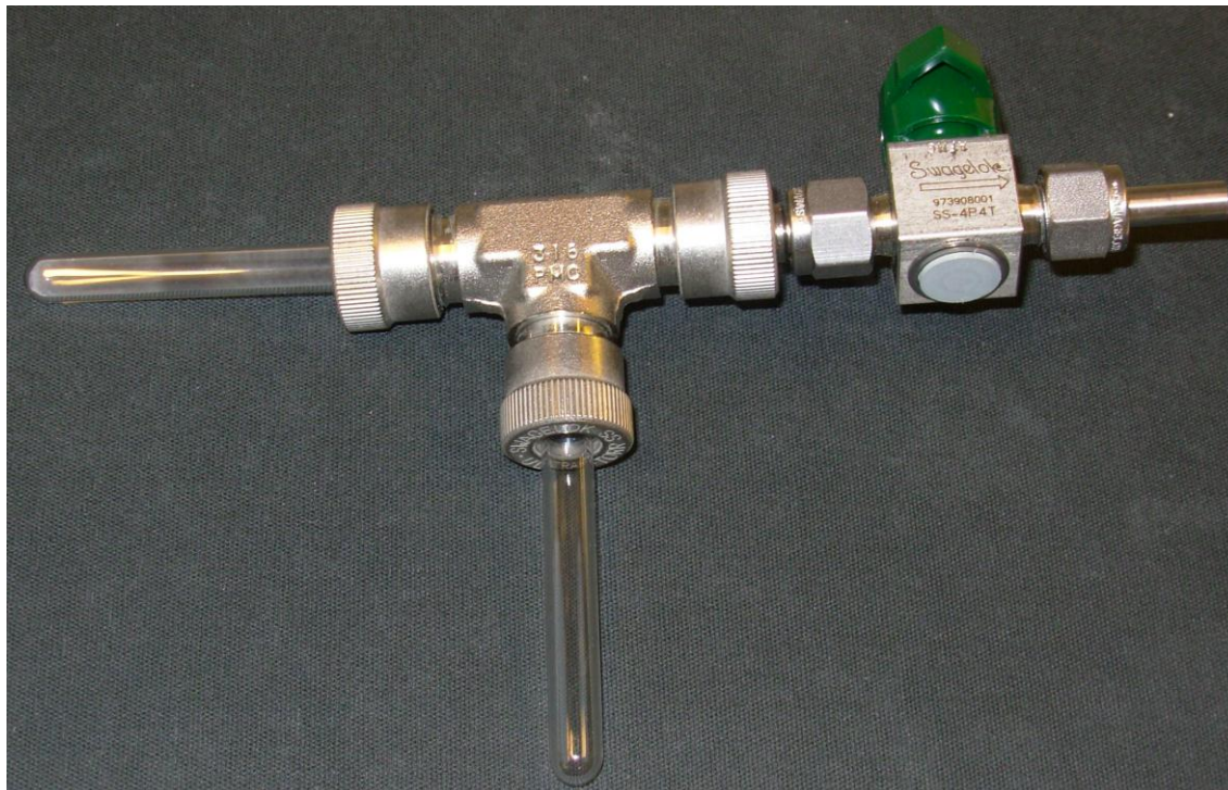
Figure 4.8 \text{CO}_2 gas container (rig) filled with iron catalyst.
