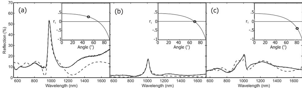
**Figure 3.1.** Experimental reflection spectra of the photonic-crystal slab for 3 angles of incidence: 50° (a), 70° (b) and 80° (c). The dashed lines are fits using the model discussed in the text. The insets show the reflection coefficient  $r_1$  for an interface of air and  $n_{\text{eff}} = 2.5$ , as function of angle of incidence. The circles indicate the angle of the measurement.
