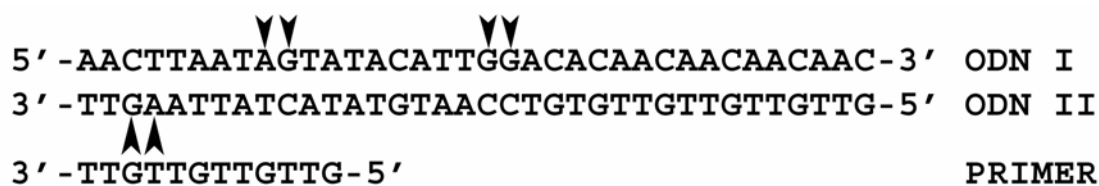
Figure 4.2 Nucleobase sequences of ODN I, ODN II and the primer used for the binding experiments. The known preferential binding sites of cisplatin are indicated by arrows.
