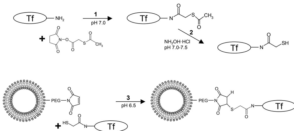
**Figure 2:** Reaction scheme of the thiolation of Tf with N-succinimidyl-S-acetylthioacetate (SATA, step 1), the activation of thiolated Tf with hydroxylamine HCl (step 2) and the conjugation of Tf to liposomes, bearing maleimide-PEG-DSPE (step 3).
