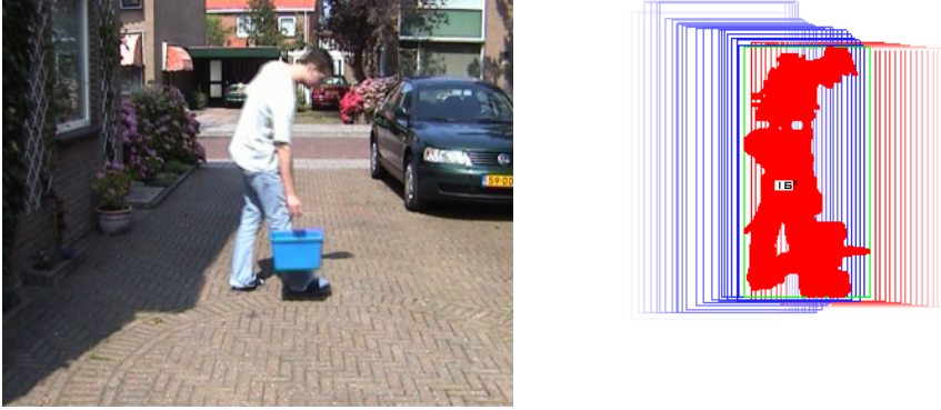
Figure 10.3: One frame from a sequence where someone leaves an object behind, together with the object tracking results.
