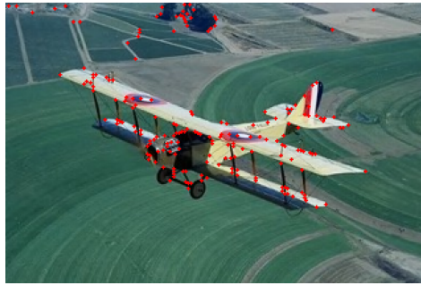
Figure 5.4: An image with the output of the Harris corner detector.
