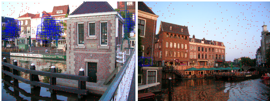
Figure 6.7: Tree detection with neural network classification.
