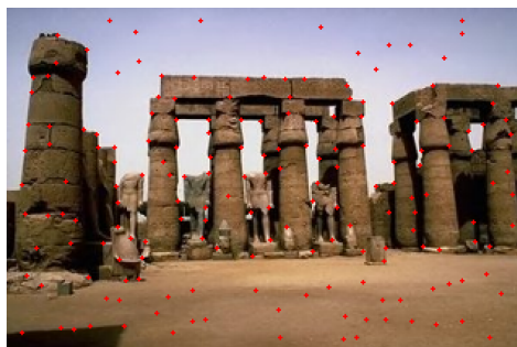
Figure 5.12: An image with the output of the MOD interest point detector.
