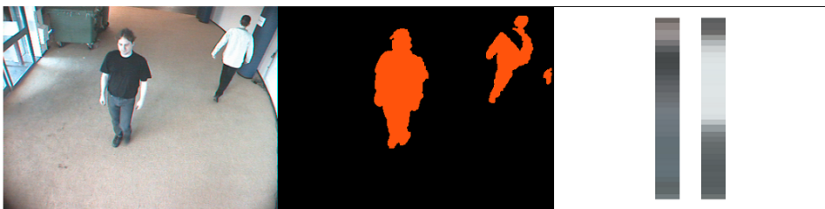
Figure 9.4: Output of the motion detection algorithm: blobs and their color models.
