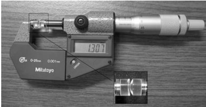
Fig. 1 The acrylic phantom joint connected to a micrometer
