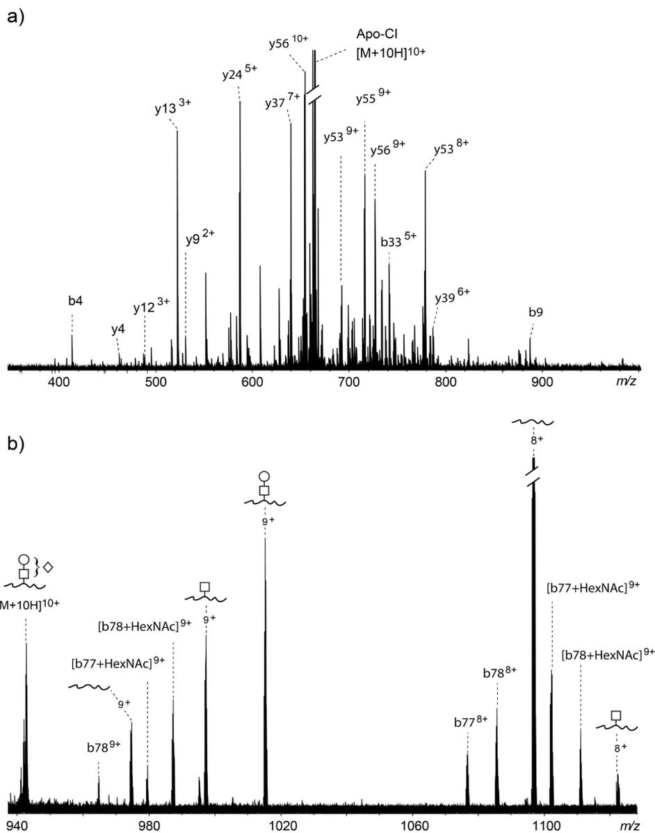
**Figure 2.** Enlarged parts of the CID spectra of Apo-CI (A) and Apo-CIII<sub>1</sub> (B) obtained with direct infusion ESI-FT-ICR-MS/MS of serum samples that were purified by RPC4 cartridge-based SPE. In both cases, the  $[M+10H]^{10+}$  precursor ion was selected in the quadrupole (Q) to perform MS/MS experiments. In the MS/MS spectrum of Apo-CIII<sub>1</sub> (B) all fragment ions lack the O-glycan, unless indicated explicitly.
