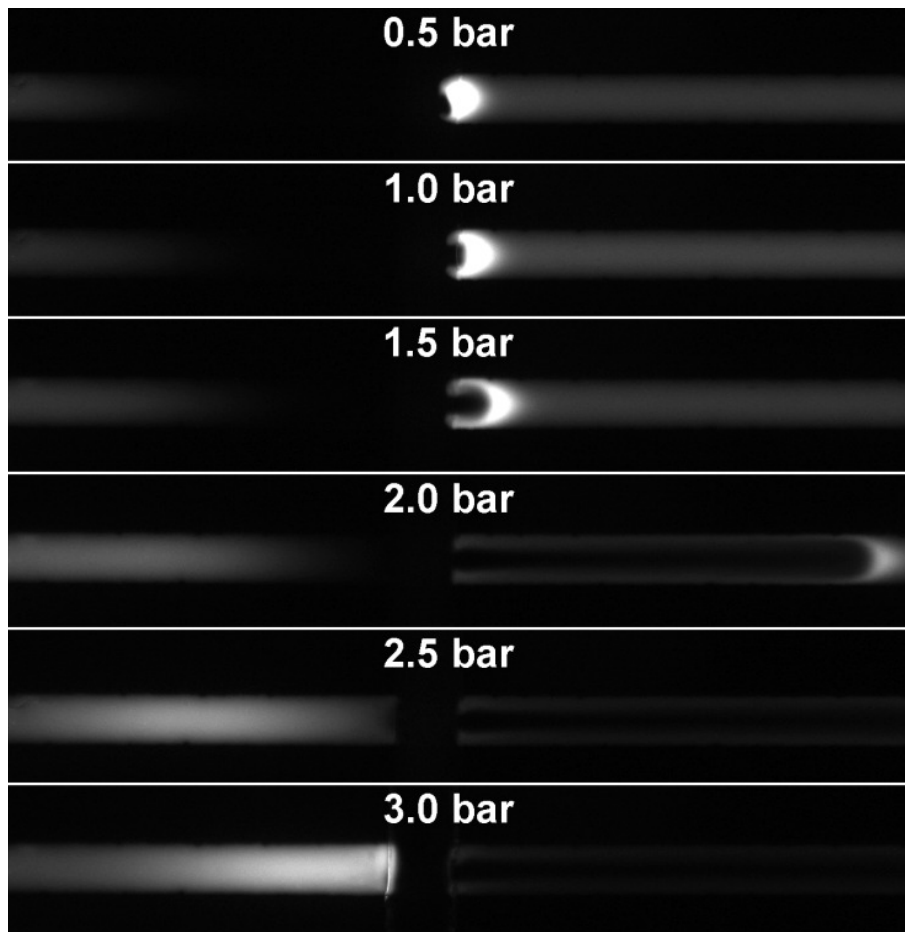
Figure 3. Concentration polarization regimes at different valve pressures in a 2.0 mmol/L lithium carbonate solution containing 40 \mu\text{mol/L} fluorescein. A constant current of 100 \mu\text{A} was applied. Images were taken 20 s after valve closure.
