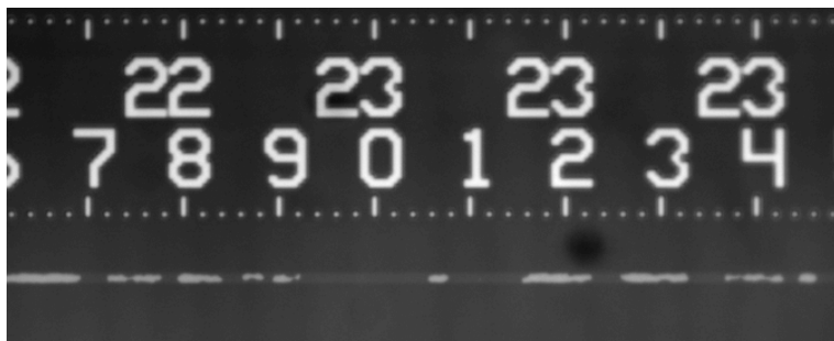
Figure 3.4 Brightfield image of bubbles in a 50 nanometer deep channel, visible as brighter regions, formed during ITP, during ITP at 500 V. in the 50 nm deep channel.
