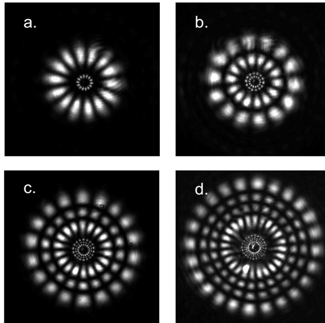
**Figure 8.2:** Measured intensity profiles of modes on the bifocal mirror for “fixed cavity length” within a free spectral range. The half-symmetric resonator ( $R = 14$  mm) is operated close to instability at a cavity length of  $L = 13.88$  mm. The modes shown are (a)  $LG_{7,0}$ , (b)  $LG_{7,1}$ , (c)  $LG_{9,2}$ , and (d)  $LG_{12,3}$ . The area shown is  $1.7 \times 1.7 \text{ mm}^2$  on the bifocal mirror. Note the smaller copy of the intensity profile inside.
