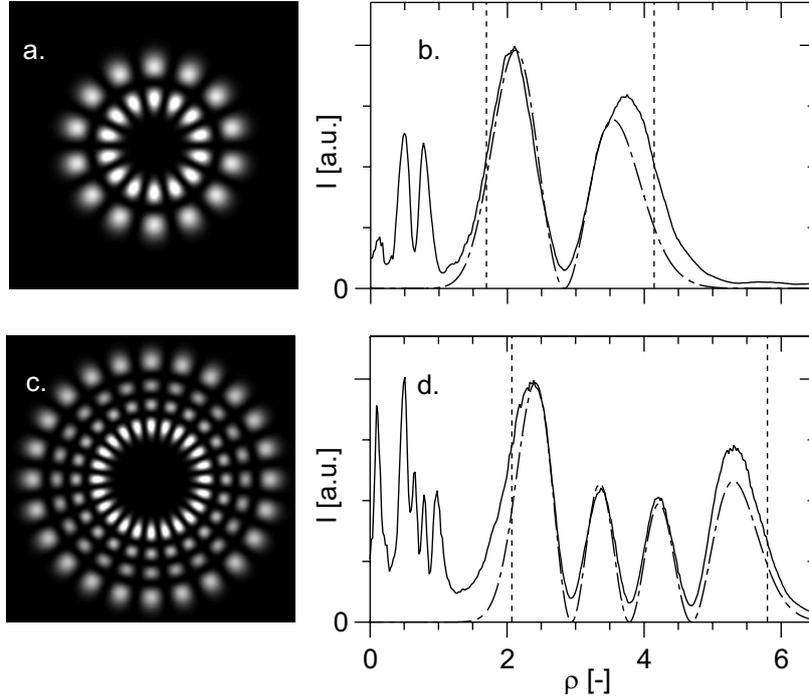
**Figure 8.3:** Calculated intensity profiles of the (a)  $LG_{7,1}$  and (c)  $LG_{12,3}$  modes. The accompanying calculated (dot-dashed lines) and measured (solid lines) rotationally-averaged intensity profiles are shown in (b) and (d). Note the inner copy of the measured intensity profiles. The vertical dotted lines indicate the classical turning points of the modal ray.  $\rho$  is the dimensionless transverse position.
