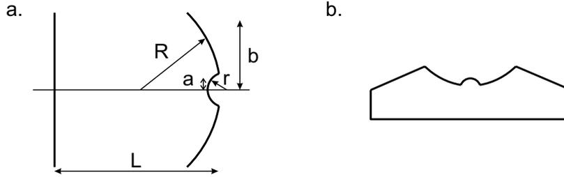
**Figure 8.1:** (a) Our cavity configuration, operated at  $L = 13.88$  mm, comprises a flat mirror and a bifocal mirror. The dimensions of the bifocal mirror are  $R = 14$  mm,  $r = -3$  mm,  $a = 100$   $\mu$ m, and  $b = 1$  mm. (b) Sketch of the bifocal mirror, where the concave and convex inner part form the mirror. The conical outer part makes the handling of the mirror easier and prevents light to be scattered back into the cavity.
