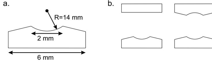
**Figure 7.1:** (a) Sketch of the diamond-machined substrate, where the concave part is the actual mirror. The conical outer part prevents this part from reflecting light back into the inner part via reflection by the opposite mirror. (b) The half-symmetric and the symmetric cavity configuration.
