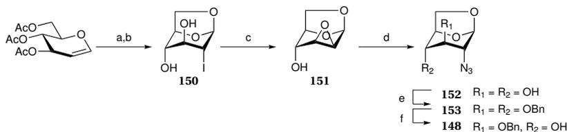
**Reagents and conditions:** a) MeOH/H<sub>2</sub>O/Et<sub>3</sub>N; b) (1) (Bu<sub>3</sub>Sn)<sub>2</sub>O,  $\Delta$ , ACN; (2) I<sub>2</sub>, DCM, 4 °C; c) NaHCO<sub>3</sub>, DMF/H<sub>2</sub>O, 98% over three steps; d) NaN<sub>3</sub>, DMF/H<sub>2</sub>O, 120 °C, 52%; e) BnBr, NaH, DME, 0 °C, 80%; f) TiCl<sub>4</sub>, DCM, 75%.
