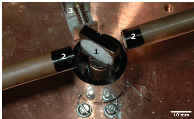
Figure 7.5 — The dust-filled target (1) is the square piece at the center of the collision space. To the left and right are the two guiding tubes (2) within which the dust aggregates are accelerated. Above center, the solenoid release mechanism (3) for the target is visible (see Section 7.2.4).
