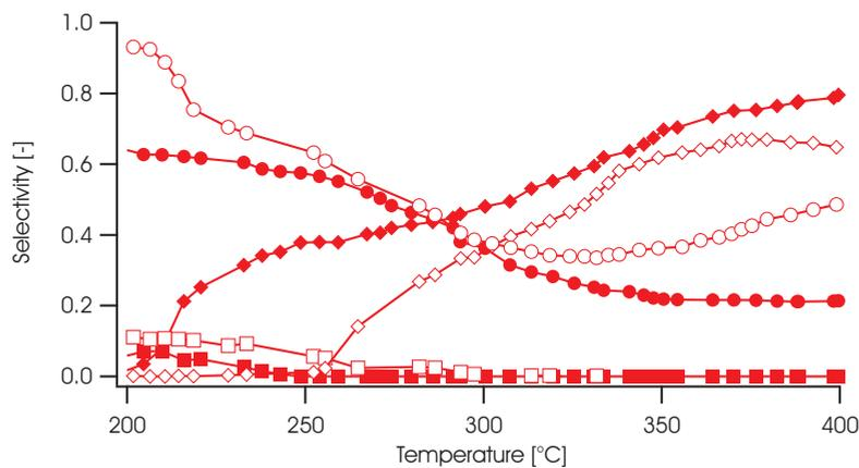
Figure 3.12: Product distribution vs temperature during NH<sub>3</sub> oxidation over Au/CeO<sub>x</sub>/Al<sub>2</sub>O<sub>3</sub> (full symbols) and Au/Li<sub>2</sub>O/CeO<sub>x</sub>/Al<sub>2</sub>O<sub>3</sub> (open symbols): Selectivity to N<sub>2</sub>O(◇), Selectivity to N<sub>2</sub> (●), Selectivity to NO(■) [12].
