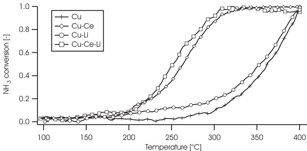
Figure 3.3: Effect of addition of  $\text{Li}_2\text{O}$ ,  $\text{CeO}_x$  and  $\text{Li}_2\text{O} + \text{CeO}_x$  on the  $\text{NH}_3$  conversion over  $\text{Cu}/\text{Al}_2\text{O}_3$  catalysts,  $\text{NH}_3:\text{O}_2 = 1$ .
