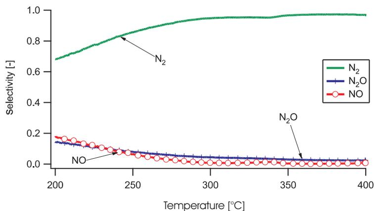
Figure 3.8: Selectivity of the Ag/Li<sub>2</sub>O/CeO<sub>x</sub>/Al<sub>2</sub>O<sub>3</sub> catalyst, NH<sub>3</sub>:O<sub>2</sub> = 1.
