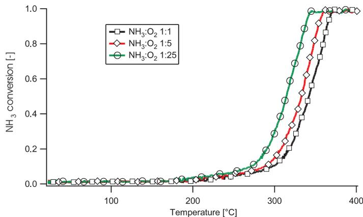
Figure 3.5: NH<sub>3</sub> conversion of Ag/Al<sub>2</sub>O<sub>3</sub> catalyst for different NH<sub>3</sub>:O<sub>2</sub> ratios.
