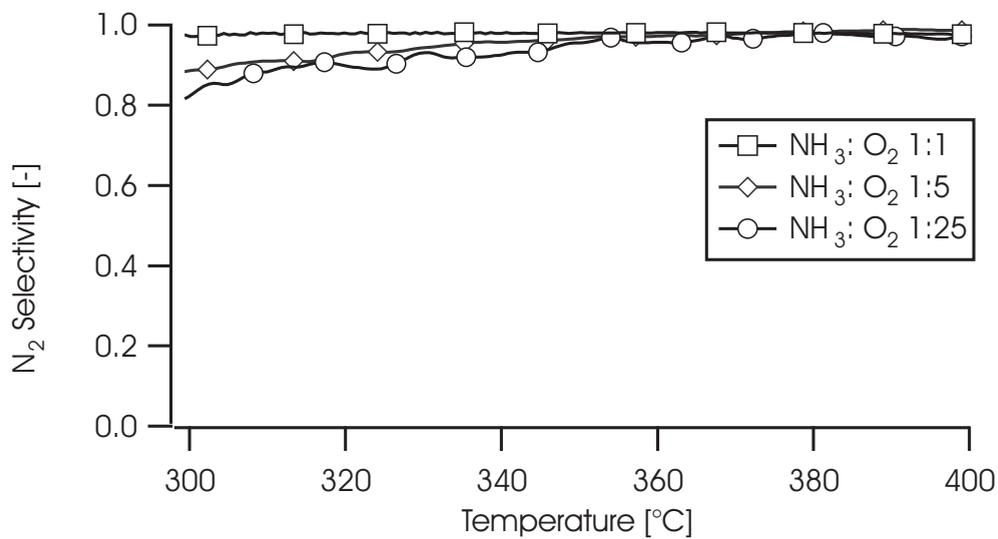
Figure 3.2: N<sub>2</sub> selectivity of the Cu/Al<sub>2</sub>O<sub>3</sub> catalyst for different NH<sub>3</sub>:O<sub>2</sub> ratios.
