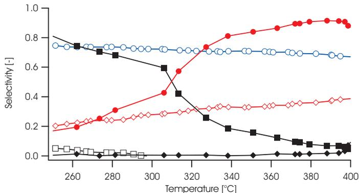
Figure 3.10: Product distribution vs temperature during  $\text{NH}_3$  oxidation over  $\text{Au}/\text{Al}_2\text{O}_3$  for two different reactant ratios. Full symbols:  $\text{NH}_3:\text{O}_2 = 1:1$ , open symbols:  $\text{NH}_3:\text{O}_2 = 1:10$ . Selectivity to  $\text{N}_2\text{O}$  (◆), Selectivity to  $\text{N}_2$  (●), Selectivity to  $\text{NO}$  (■) [12].
