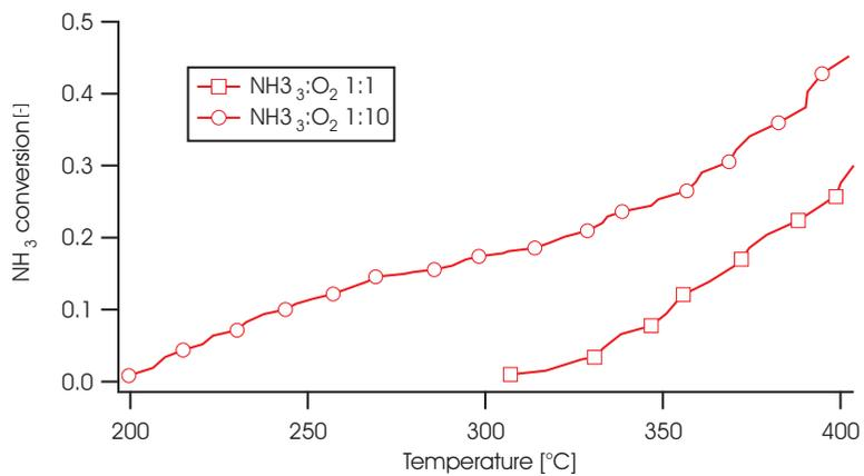
Figure 3.9: NH<sub>3</sub> conversion of Au/Al<sub>2</sub>O<sub>3</sub> catalyst for different NH<sub>3</sub>:O<sub>2</sub> ratios [12].
