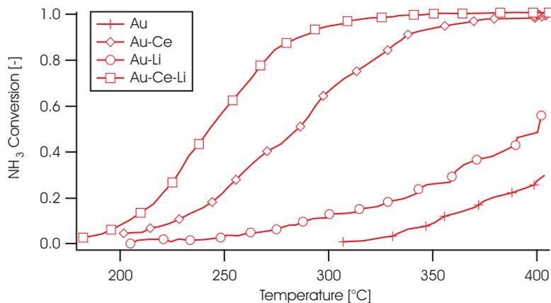
Figure 3.11: Effect of addition of Li<sub>2</sub>O, CeO<sub>x</sub> and Li<sub>2</sub>O + CeO<sub>x</sub> on the NH<sub>3</sub> conversion of Au/Al<sub>2</sub>O<sub>3</sub> catalysts [12].
