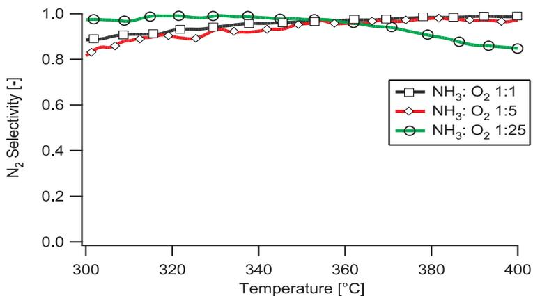
Figure 3.6: N<sub>2</sub> selectivity on the Ag/Al<sub>2</sub>O<sub>3</sub> catalyst for different NH<sub>3</sub>:O<sub>2</sub> ratios.
