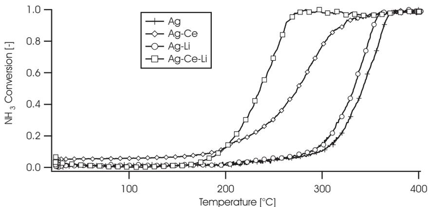
Figure 3.7: Effect of addition of Li<sub>2</sub>O, CeO<sub>x</sub> and Li<sub>2</sub>O + CeO<sub>x</sub> on the NH<sub>3</sub> conversion of Ag/Al<sub>2</sub>O<sub>3</sub> catalysts, NH<sub>3</sub>:O<sub>2</sub> = 1.
