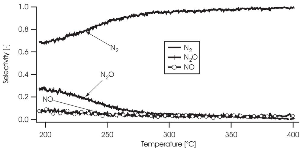
Figure 3.4: Selectivity of the  $\text{Cu}/\text{Li}_2\text{O}/\text{CeO}_x/\text{Al}_2\text{O}_3$  catalyst,  $\text{NH}_3:\text{O}_2 = 1$ .
