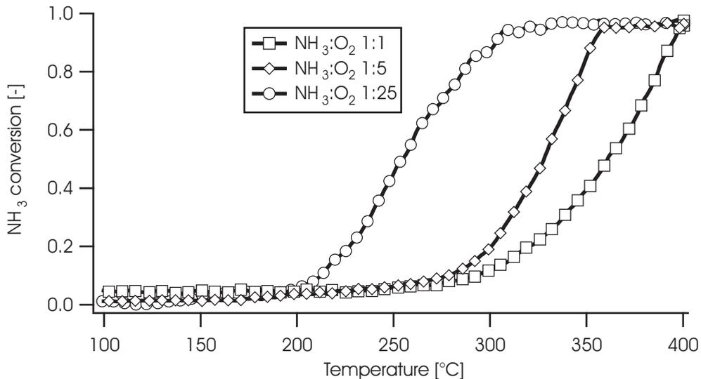
Figure 3.1: NH<sub>3</sub> conversion on Cu/Al<sub>2</sub>O<sub>3</sub> catalyst for different NH<sub>3</sub>:O<sub>2</sub> ratios.
