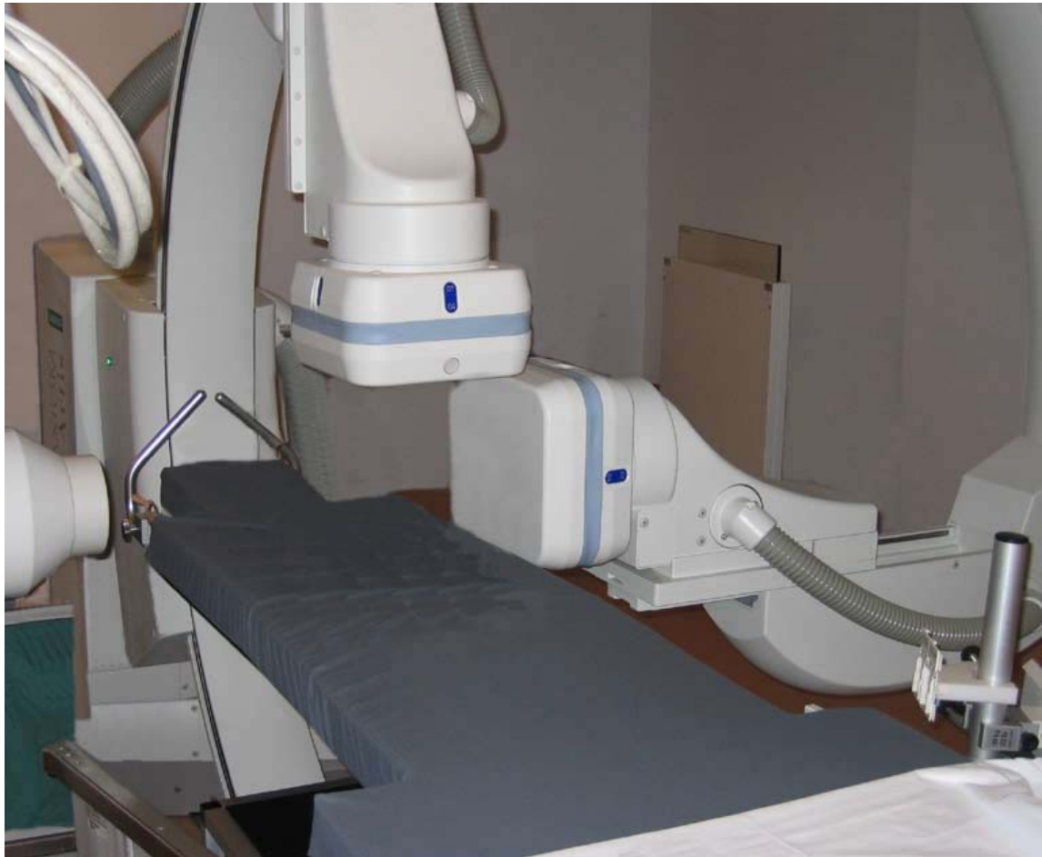
Figure 1. FRSA set-up consisting of two C-arms with digital flat panel Roentgen detectors (Siemens Axiom Artis dBc imaging system, Siemens AG, Erlangen, Germany).
