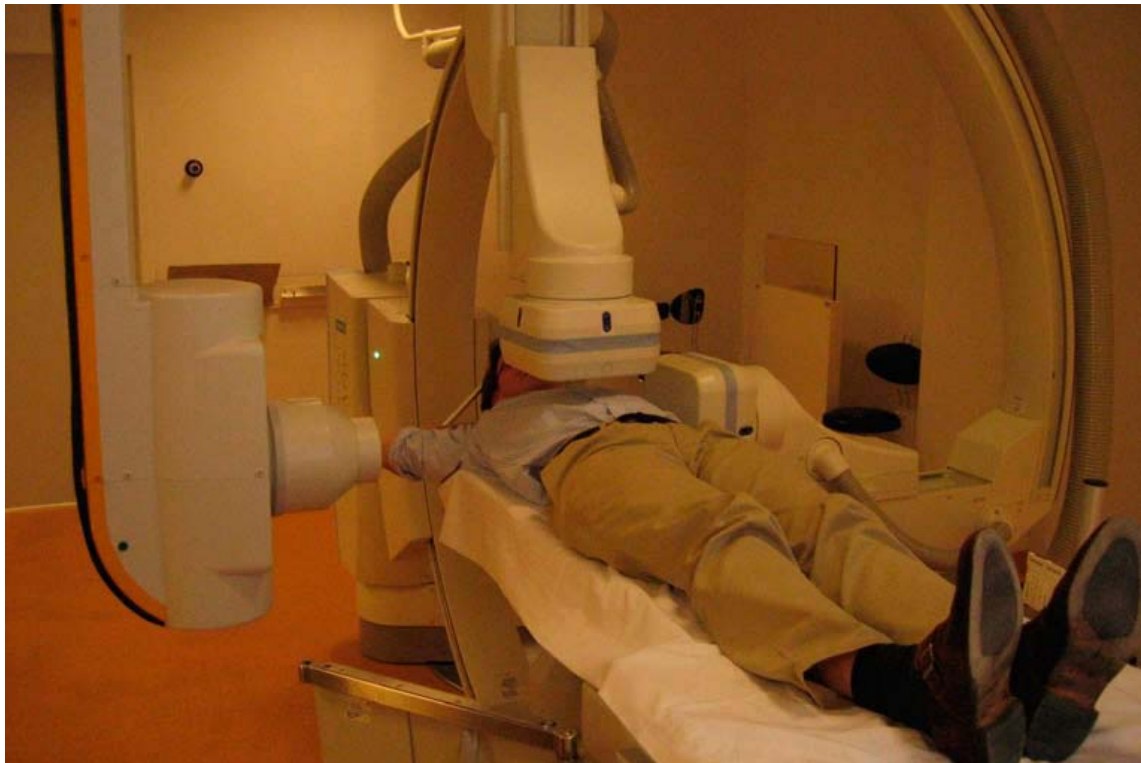
Figure 2. Clinical set-up of the bi-plane fluoroscope
