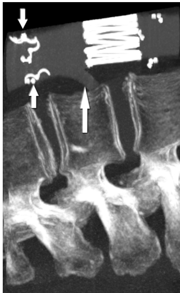
Figure 4. 3D maximum intensity projection of the CT image of the model. Short arrow lower left: tantalum marker; short arrow upper left: nitinol clip; long arrow lower right: renal artery. Cranial side to the left.
