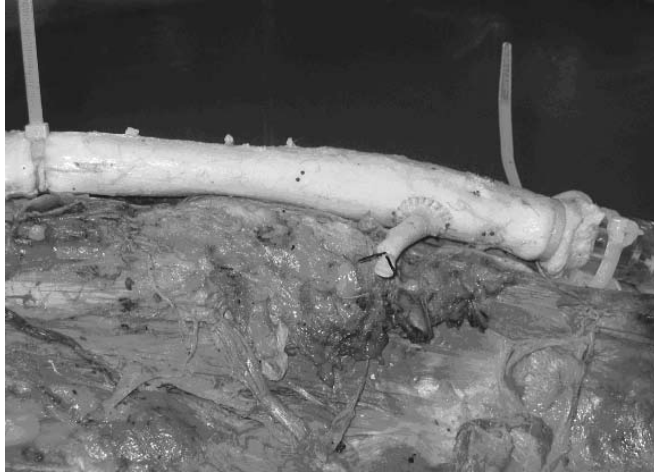
Figure 6. Pulsatile flow model. A fresh specimen of a porcine aorta was positioned ventral to a preserved human spine, complete with soft tissue. The porcine aorta replaced the human aorta. The aorta is connected to a pulsatile flow generator with physiologic flow and pressure profiles.
