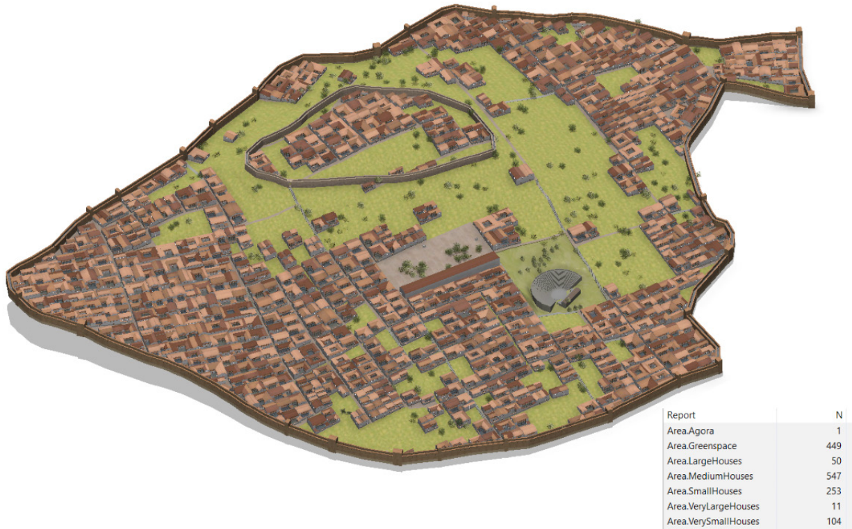
Figure 6.33 Hypothesis 4: The threshold for the terrain suitable for buildings is up to 14°, which allows 965 houses.
