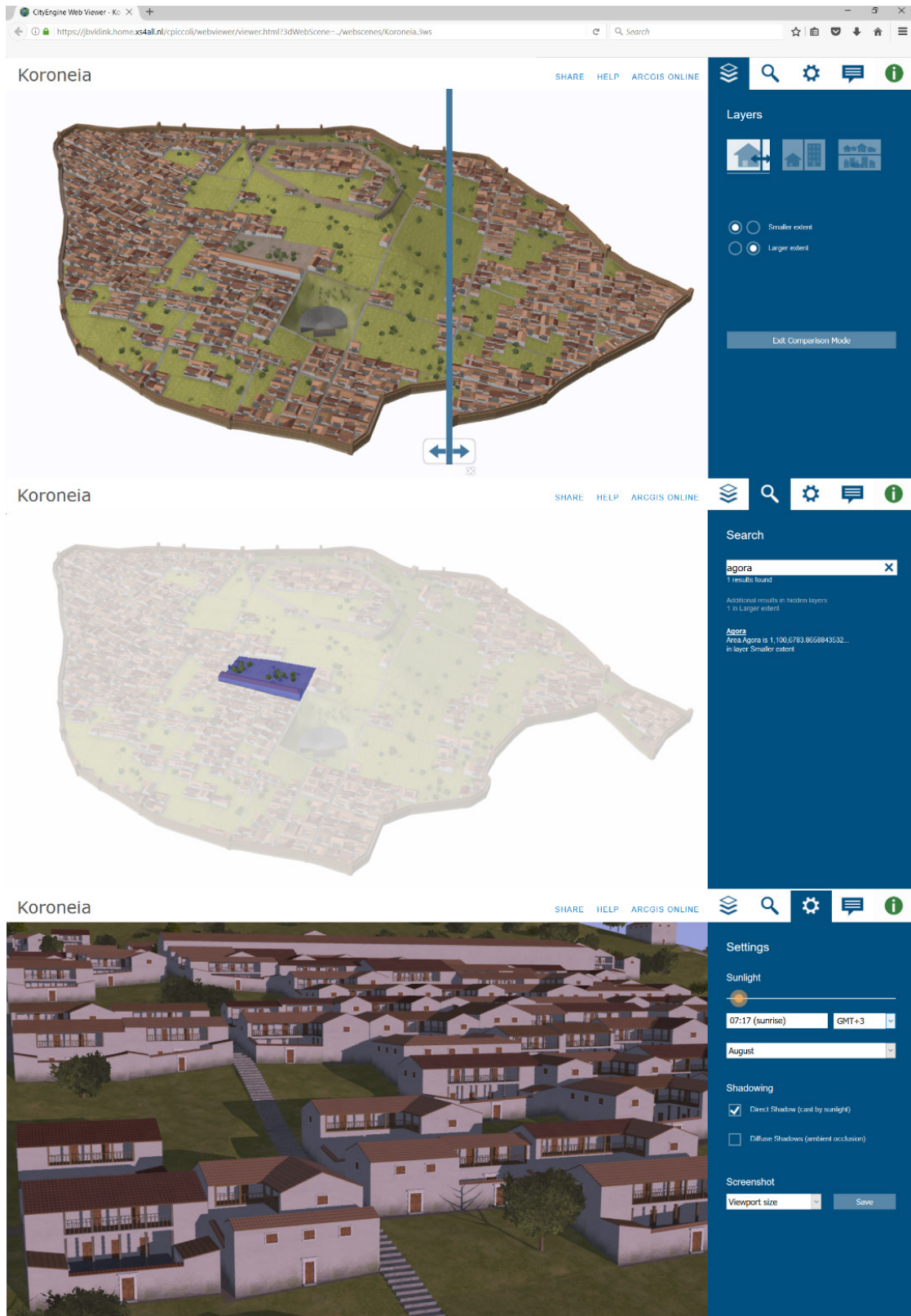
Figure 6.35 Koroneia's 3D visualization exported in the *.3ws format and viewed in the CityEngine Web Viewer: a) Alternative scenarios can be compared using the swipe view; b) buildings can be tagged so that they are easily searchable, and as shown in c) the lighting conditions can be changed to see their impact on the 3D scene.
