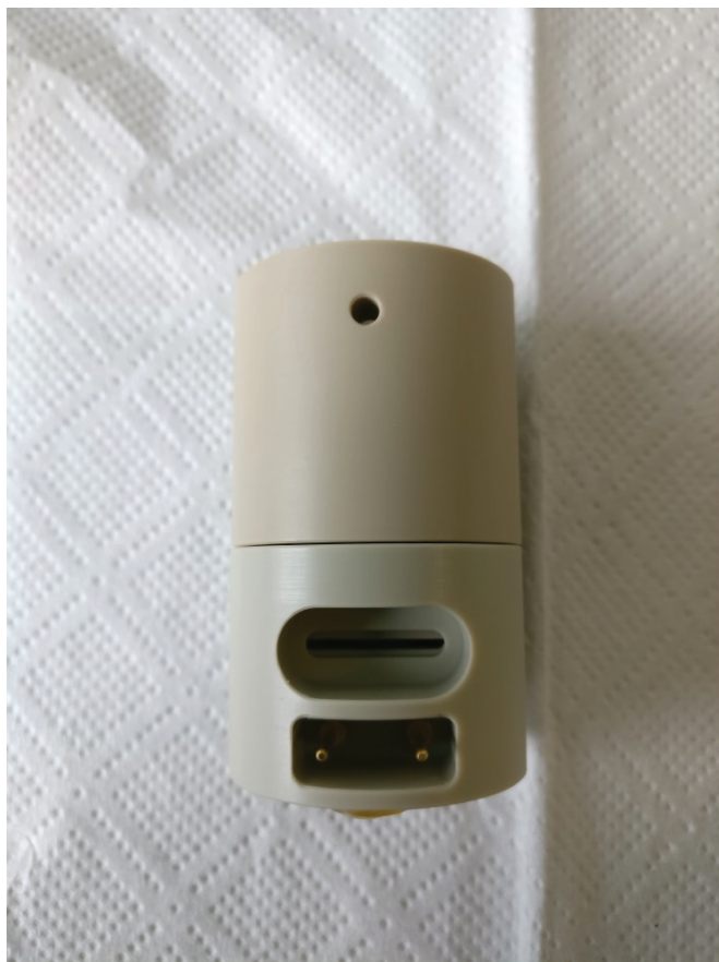
Figure B.9: Modified EQCM cell: the top part of the cell was made taller to allow for degassing of the electrolyte solution by bubbling argon. Additionally, a small hole was added to serve as a gas inlet to keep the cell under argon flow during experiments, preventing air from entering.
