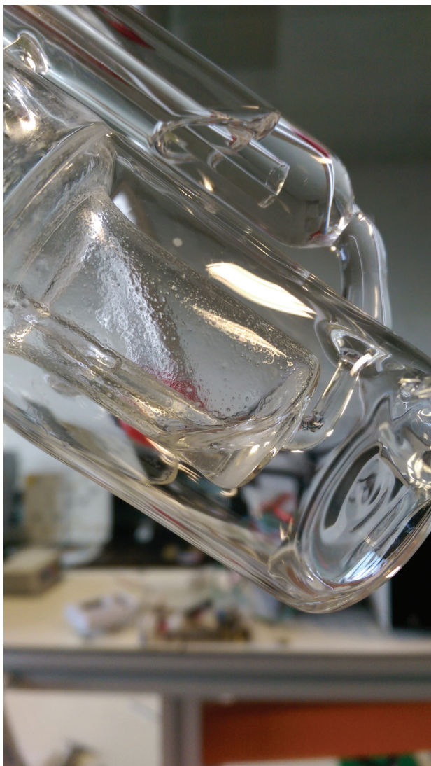
Figure C.1: Formation of solid precipitate inside the electrochemical cell during electrochemical measurements of complex 2 in 0.1 M \text{HClO}_4
